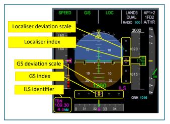
Figure 5 - Primary Flight Display with ILS (Source: Airbus)
