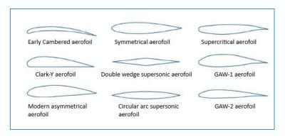
Figure 1 - Aerofoil types
