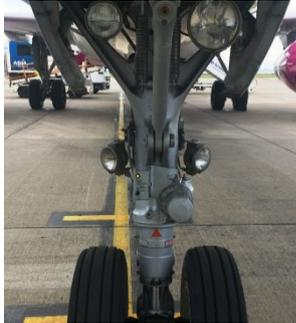
The nosewheel serves to steer during taxi. This also has the taxi and turnoff lights as well as a damper to prevent nosewheel shimmy (or vibration). On large aircraft, the mechanism for the nosewheel steering disconnection allows for towing the aircraft by cutting off any hydraulics to the steering mechanism. In addition, a centering mechanism centres the nose gear before retraction...
