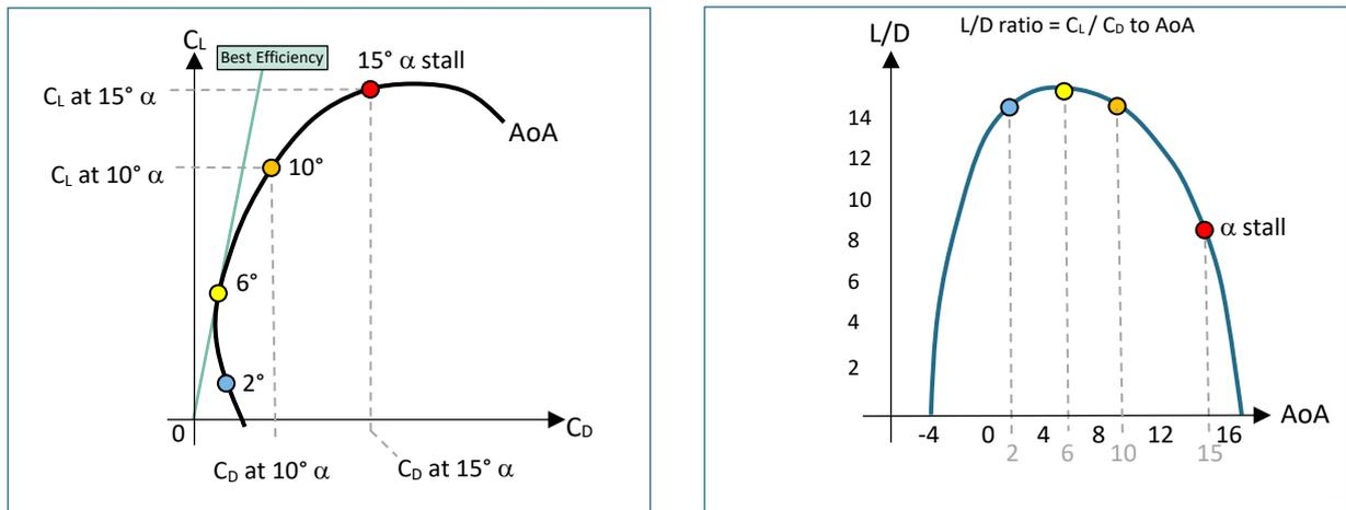
Figure 8 - Polar curve and L/D Ratio to AoA
