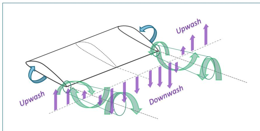
Figure 5 – Three-dimensional flow
