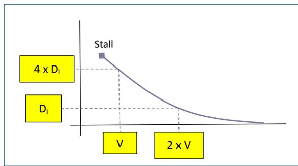
Figure 6 - Induced Drag curve
