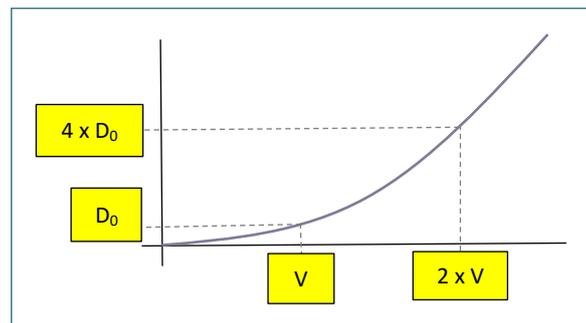
Figure 4 - Zero lift drag and speed relationship
