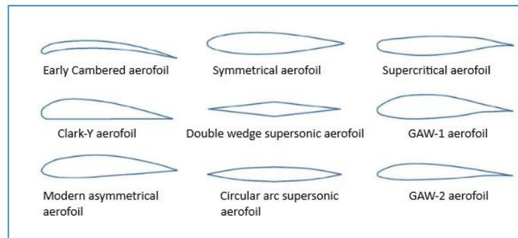
Figure 1 - Aerofoil types
